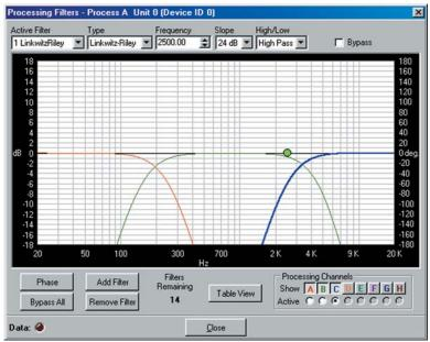
Figure 3.48. Low/Mid/High Loudspeaker Driver configuration
